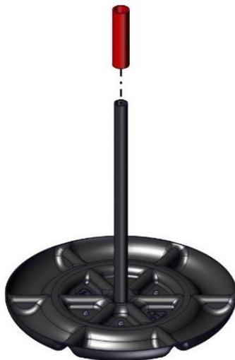
7. Add the same color Middle Tray (am-4492\_Red or Blue) to the assembly by pressing the center of the tray onto the pipe. This is Level 2.
